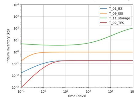
Figure 2: log plot showing the time evolution of tritium inventories in various components of the reference Helios fuel cycle
