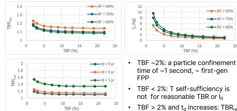
Figure 3: plots showing how  $I_0$  and TBR<sub>req</sub> change with tritium burn fraction, at different values of AF and  $t_d$
