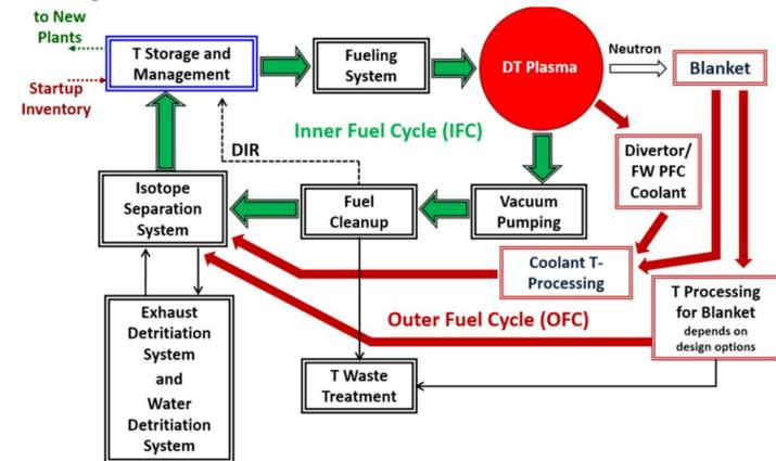
Figure 1: block diagram of ITER's fuel cycle components and T fuel flow between them.<sup>1</sup> Helios will have the same fuel cycle components and processing times, while allowing for a different blanket / divertor / first wall architecture
