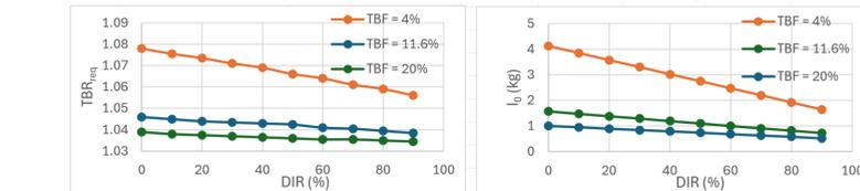
Figure 4: plot showing how  $I_0$  and TBR<sub>req</sub> change with direct internal recycling fraction and tritium burn fraction
