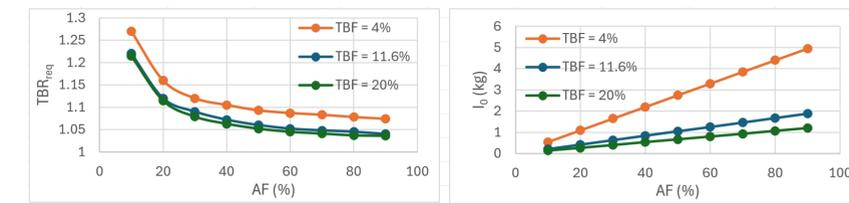
Figure 6: plot showing how  $I_0$  and TBR<sub>req</sub> change with availability factor and tritium burn fraction
