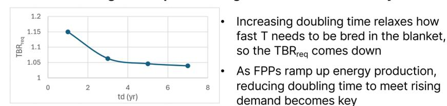
Figure 5: plot showing how TBR<sub>req</sub> changes with doubling time
