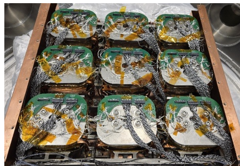
Figure 3: Canis 3x3 array with mounted Winding Pack Instrumentation Board
