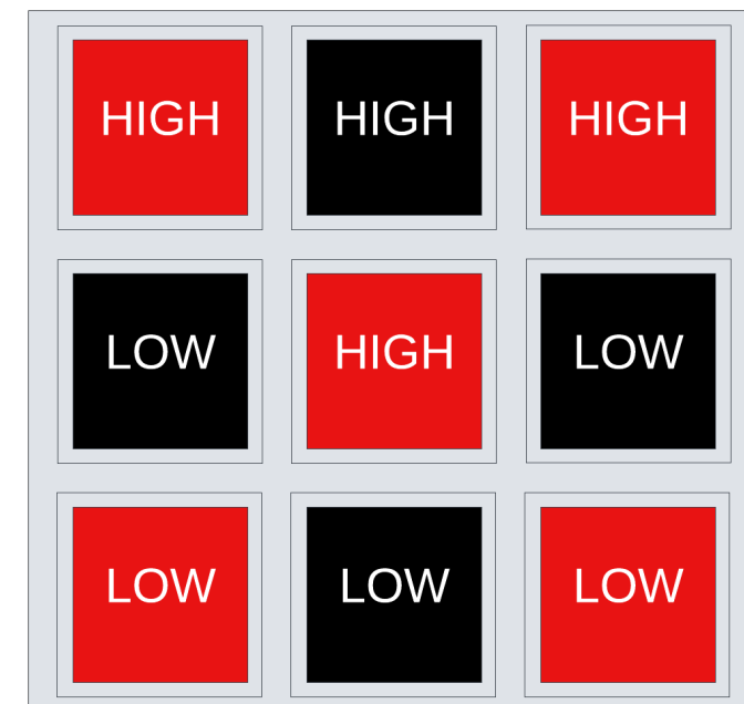
Figure 6: "Checkboard" magnet array excitation pattern, red indicated positive current flow black indicates negative current flow while HIGH/LOW designates magnet resolution
