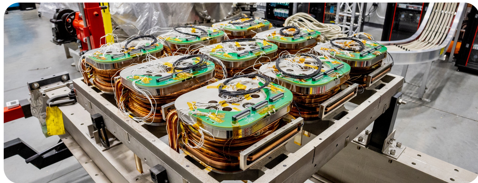
Nine fully assembled, instrumented, and validated SMI planar coil-based winding packs mounted to the Canis 3x3 magnet array gravity support assembly, awaiting installation into the Canis cryostat.
