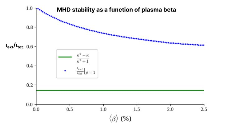
The minimum value of  $\iota_{ext}/\iota_{tot}$  is plotted . The green line is the minimum required external rotational transform from Fu et.al. [3] that guarantees vertical stability.
