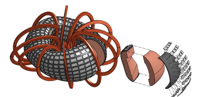
Planar coils enable easier access to the vessel where remote manipulators can remove and maintain entire sectors of the system
