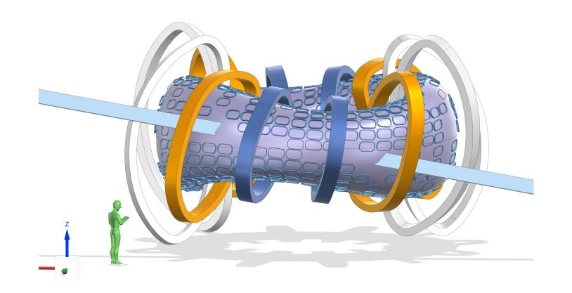
Two negative ion deuterium neutral beams (only one shown in the figure) of energy with energy of ~ 1 MeV will be injected into the deuterium plasma to generate D-D neutrons.
