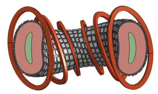
Quasi-axisymmetry provides ample room for blanket system between plasma and magnet systems
